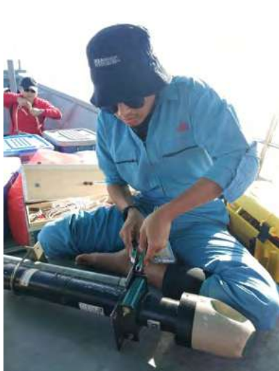
Acoustic Doppler and Current Profiler (ADCP) used to measure in-situ currents.
