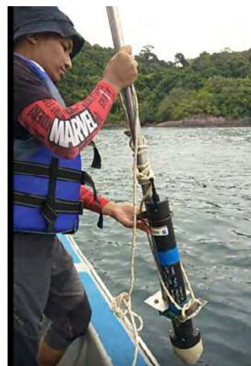
Acoustic Doppler and Current Profiler (ADCP) used to measure in-situ currents.
